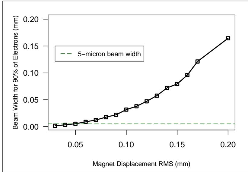
Figure 2: RMS of Beam Displacement vs. Beam Width.
