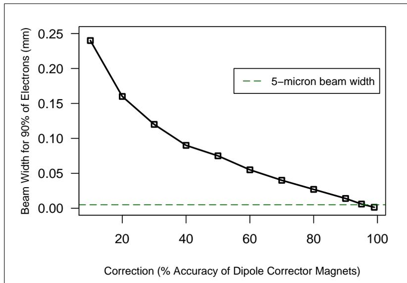
Figure 3: Correction vs. Beam Width; Magnet Displacement RMS = 0.25
