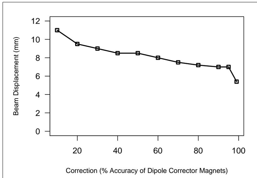
Figure 5: Correction vs. Beam Displacement; Magnet Displacement RMS = 0.25
