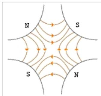
**Figure 1: Field lines of a quadrupole magnet.**
